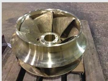
Figure 6: Impellers. Photo courtesy of Inoxyda SA.
